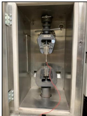
Fig. 3. Testing of ETW Specimens Within Heated Chamber
